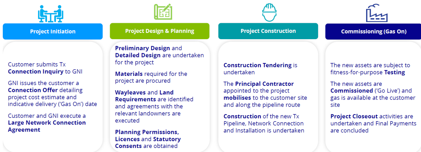
Figure 3: Connection project phases. Source: GNI.
